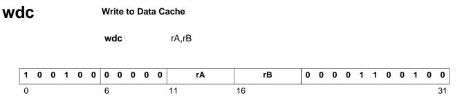
Write into the data cache tag. The register rB value is not used. Register rA contains the instruction address. Bit 30 in rA is the new valid bit.
